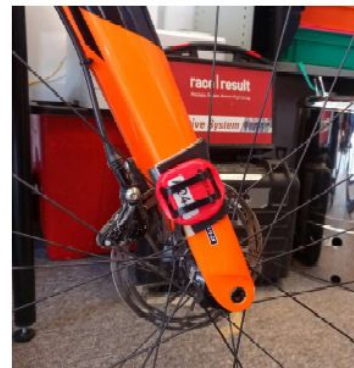
Examples of fitted timing chips on wide 'aero' forks and standard diameter bolt thru forks
